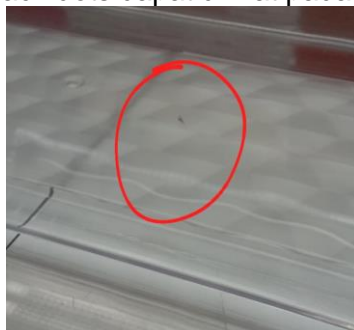
Gambar 2. Cacat Black Dots
