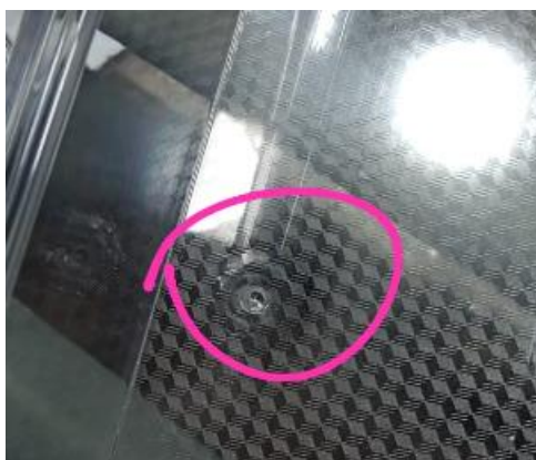
Gambar 4. Cacat Short Mold
