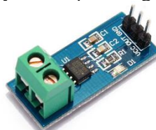
Gambar 4. Tampilan sensor arus ACS712 [2]
